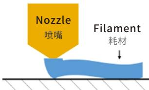
The distance between the hot bed and the nozzle is too far, you need to adjust the Z compensation, press the **arrow 2** in the figure to compensate the difference.
