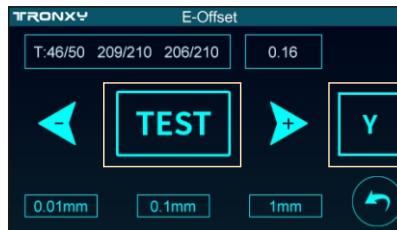
Switch to "Y", click "TEST", and start the test after the temperature reaches the requirement
