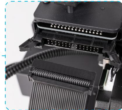
Left adapter board wiring port
