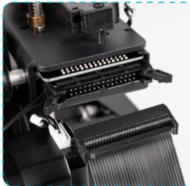
Right adapter board wiring port
