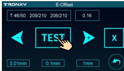
Click "Test" and start the test after the temperature reaches the requirement
