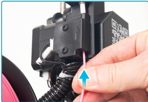
Insert the consumables from under the Filament run-out detector
