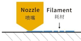
The distance between the hot bed and the nozzle is too close, you need to adjust the Z compensation, press the **arrow 1** in the figure to compensate the difference.
