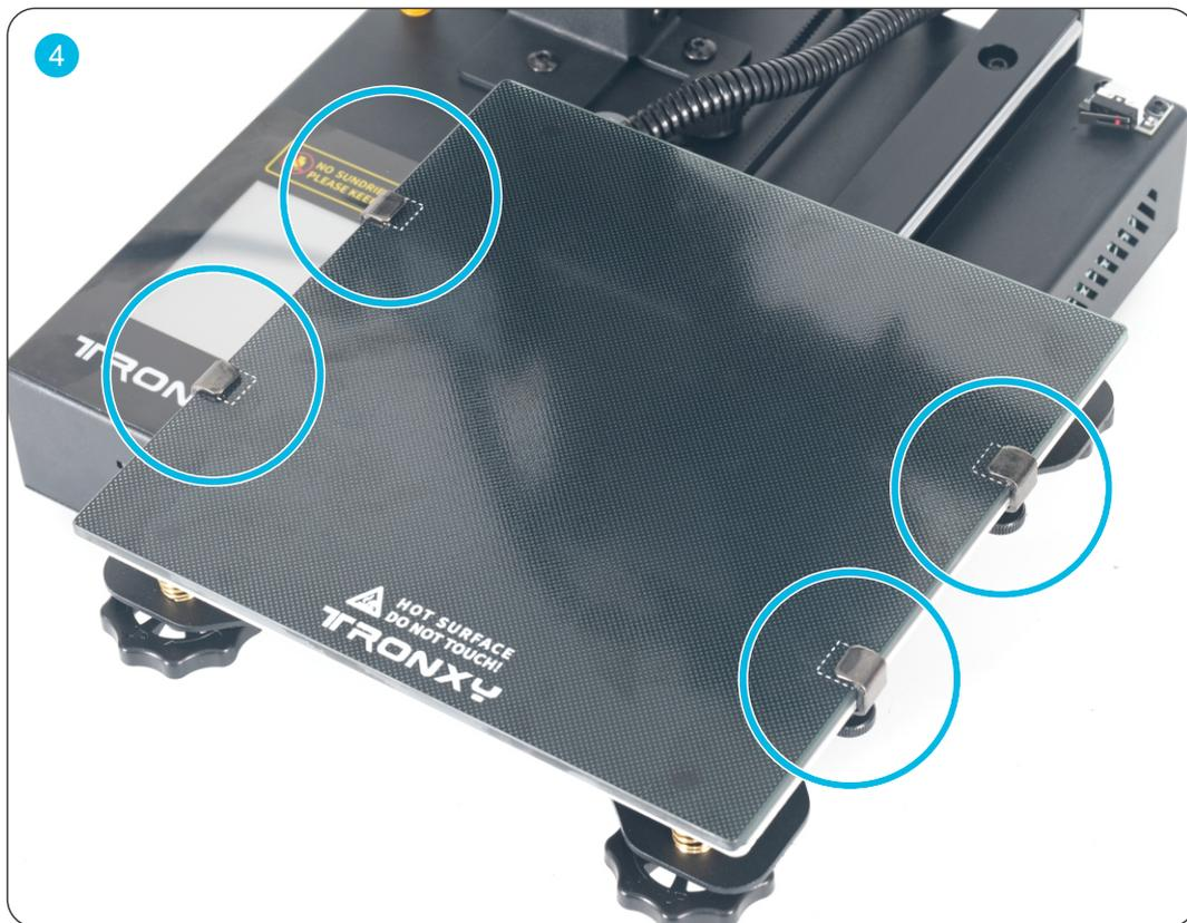
Install the remaining clips as shown in the figure
