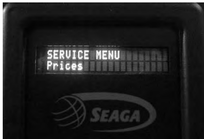
Fig. 11 – VFD Display while in Service Mode. The Prices menu is the first sub-menu.
