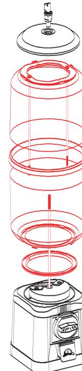
This feature, while increasing the height of the machine from the standard 16" to 23", offers an additional 95% capacity. This extended globe is great in high traffic locations. The RB23 globe is the largest capacity for the RB series machines. Easily retrofitted from standard models.
