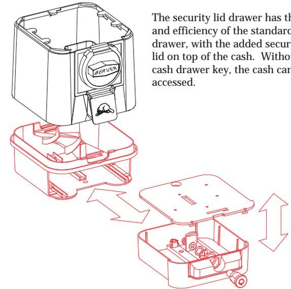
The security lid drawer has the ease and efficiency of the standard cash drawer, with the added security of a lid on top of the cash. Without the cash drawer key, the cash cannot be accessed.
