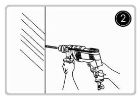
Punch holes in the wall and attach the lamp bracket.
