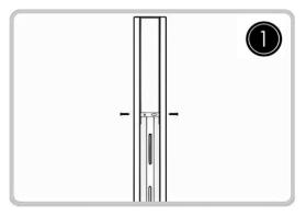
Remove the mounting bracket by loosening the screws.
