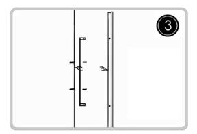
Connect wires. The junction box can be anywhere along the length of the light.
