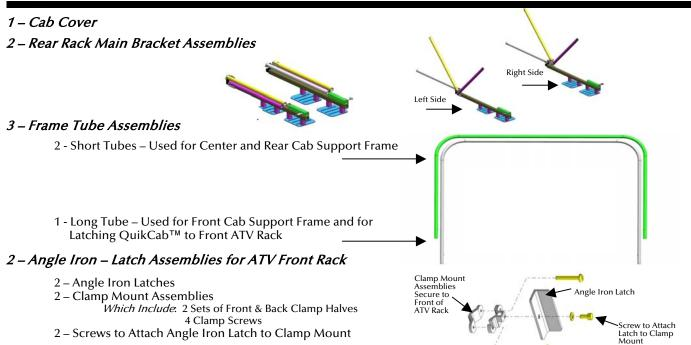
Note: Some ATV's may require other methods of attaching the latch to the front rack depending on composite and angle of rack
