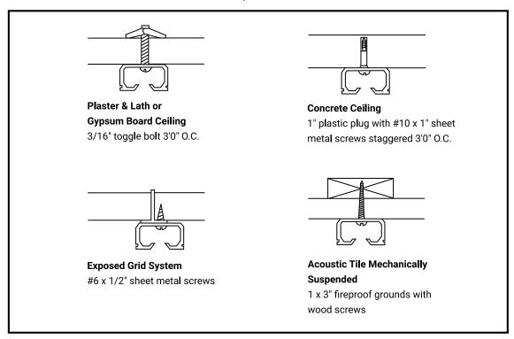
**STEP 6** - Place track (A) against ceiling and mark hole locations. If required, pre-drill holes in marked locations and install anchors, plugs, etc (will vary with ceiling type)
