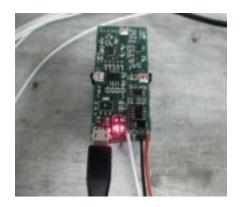
Cell Balancing, Safety, and Charge Circuit with Thermal Management
