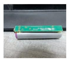
Safety Circuit with Thermal Management made for a Single Cell Battery
