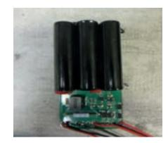
Charge, Safety, and Cell Balancing Circuit with Thermal Management and a Primary Battery Backup
