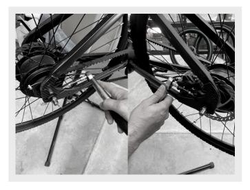
Ensure that the screw is no longer touching on both sides.
