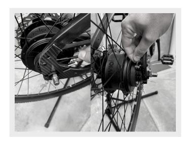
2/ Remove the bolts on both sides of the rear wheel with a 15mm spanner.
