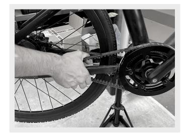
Replace the tire onto the rim, starting with positioning the Presta valve attachment. Make sure the tire is spinning in the right direction.
