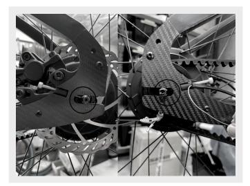
5/ Check that tension in the belt has been removed by squeezing the belt.
