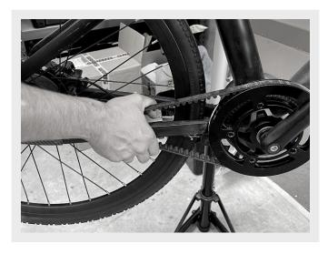
Gently remove the carbon belt using a plastic tire lever.
