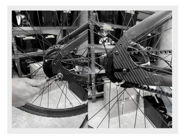
Unscrew the belt tensioner on both sides with a 5mm allen key.
