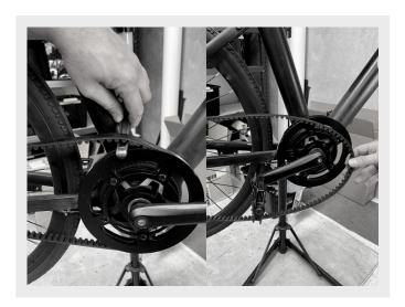
7/ Firmly girp the bike frame and pull the rear wheel backwards to remove.
