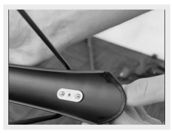
Insert the front fenders above the front wheel through the rear side of the fork and secure it by washer and the centre bolt B1 with '10' Spanner. (do not tighten them)
