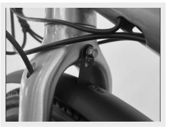
3/ Secure the stay using S2 screws on the either side of the wheels on the fork using the 4mm allen key (supplied with your e-Bike)
