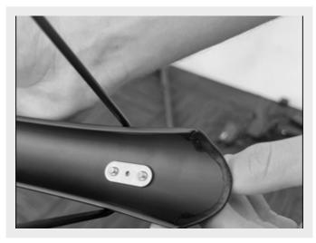
2/ Insert the rear fenders above the rear wheel through the seat stay and secure it by the washer & S3 screw with 4mm allen key. (do not tighten them)
