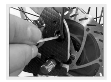
Adjust the fender to the right position by keeping a good clearance with the wheel and tighten all the screws.
