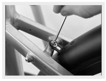
Secure the Stay using S4 screws (on your E-bike) on the either side of the wheels near the axel using the 4mm allen key (supplied with your e-Bike)
