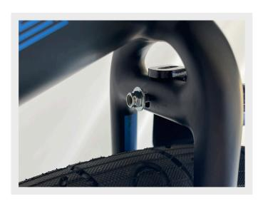
3/ Tighten completely using a 4mm hex key.
