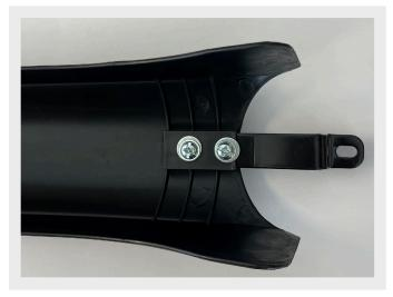
Use the large hex socket screw and a washer to attach the rear fender to the bike as shown below.
