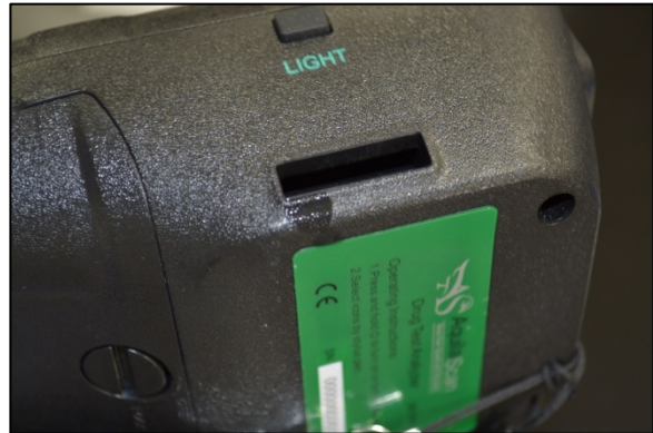
Figure 69. Saliva observed from the AquilaScan analyzer after leaking from the test cassette.
