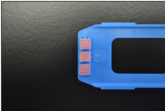
Figure 26. The DrugWipe 5S sample collector uses three thin pink colored pads to collect sample.
