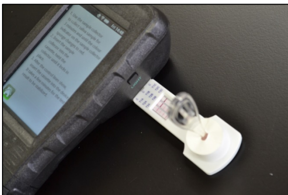
Figure 64. Once the control lines have formed the test cassette is inserted into the side of the analyzer.
