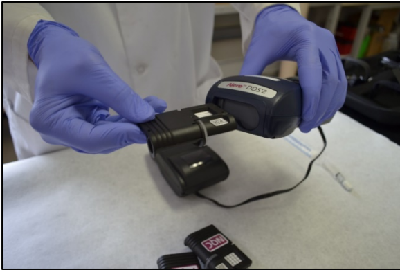
Figure 44. The test cassette is inserted into the bottom of the DDS2.
