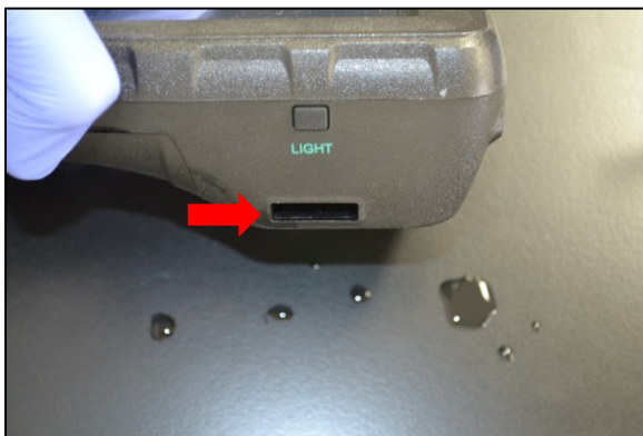
Figure 70. Saliva observed from the AquilaScan analyzer after leaking from the test cassette.
