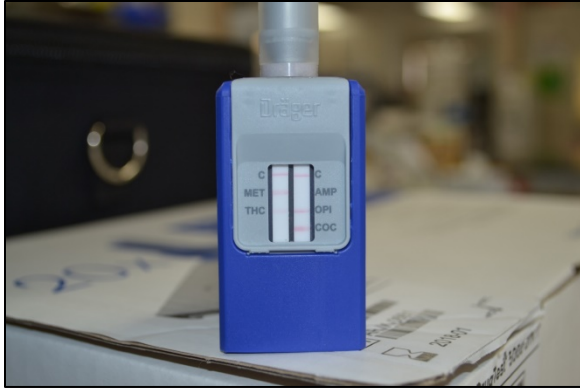
Figure 18. Completed test. The appearance of a line no matter how faint indicates a negative test. The absence of a visible line is indicative of a positive. This example is positive for amphetamine.
