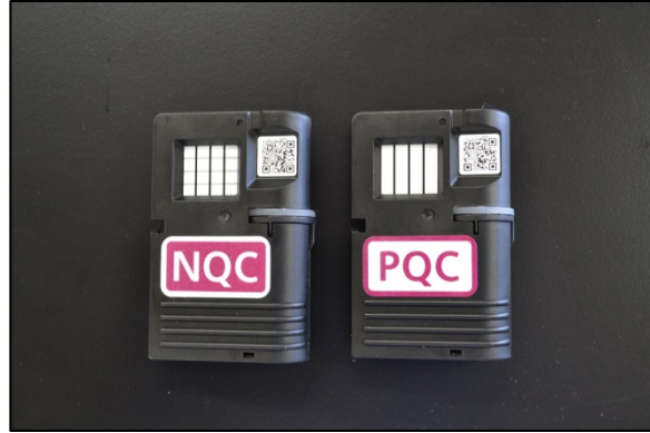
Figure 43. The DDS2 comes with a set of external quality control test cassettes.
