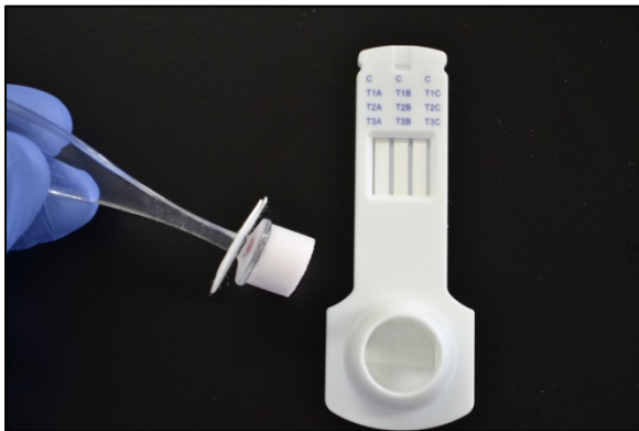
Figure 62. Once enough sample has been collected and the bar code scanned a paper splash guard is slid onto the base of the sample collector.
