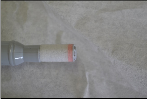
Figure 12. A pink line is visible on the sample collector before sampling.
