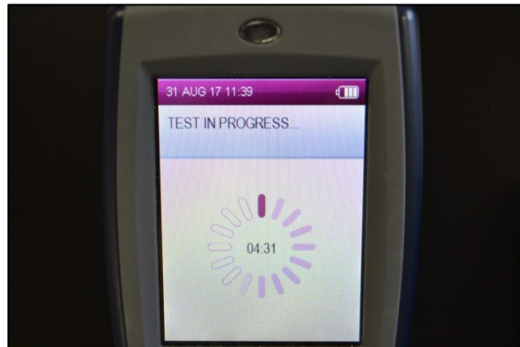
Figure 47. The DDS2 is completely automated. Testing begins automatically when the sample collector is fully inserted into the test cassette already in the analyzer.
