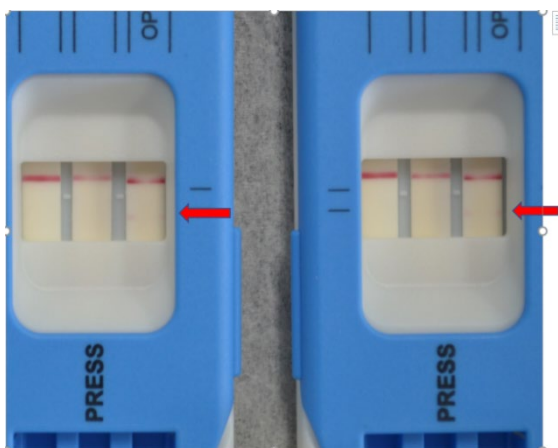
Figure 2. Faint or incomplete lines for the opiate test (indicated by the red arrow) on two test cassettes that were interpreted differently by the DrugRead analyzer.
