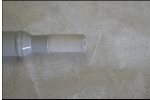
Figure 13. The pink indicator disappears after collecting sufficient sample.
