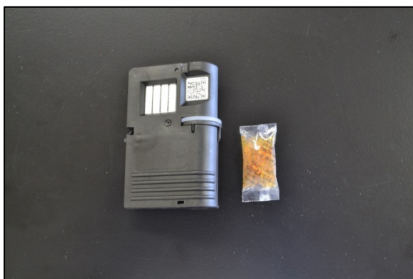
Figure 40. The DDS2 test cassette comes with a color changing desiccant. If it is yellow, testing may proceed; if it is green, the test cassette should be discarded.
