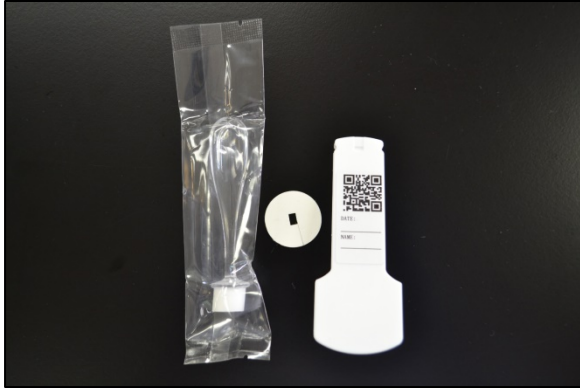
Figure 54. The back of the AquilaScan test cassette includes a bar code to be scanned by the analyzer to determine testing and whether the test kit is expired.
