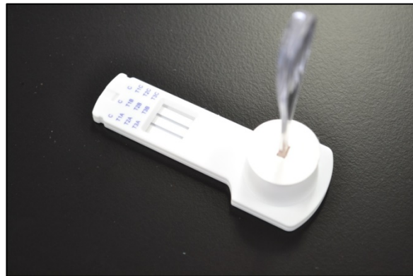
Figure 63. The sample collector is then snapped into the test cassette and twisted compressing the sponge and delivering sample.
