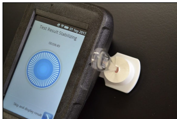
Figure 65. Once the test cassette is inserted into the analyzer a five-minute timer is automatically started.
