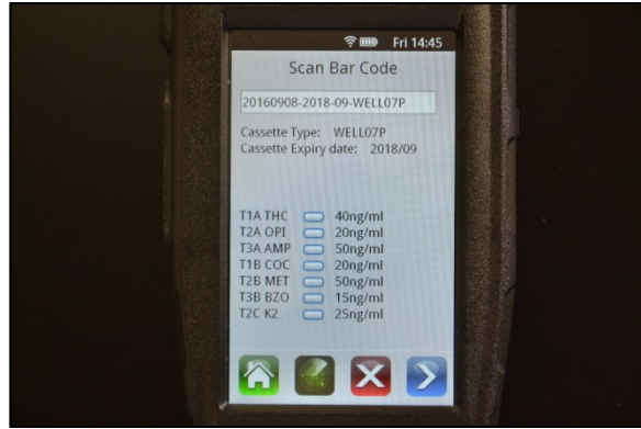
Figure 61. After scanning the bar code, the analyzer displays the testing included on the cassette as well as the cutoffs.
