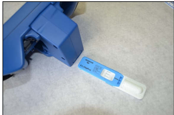
Figure 29. Resting horizontal and level the DrugWipe 5S test cassette is inserted into the DrugRead analyzer.
