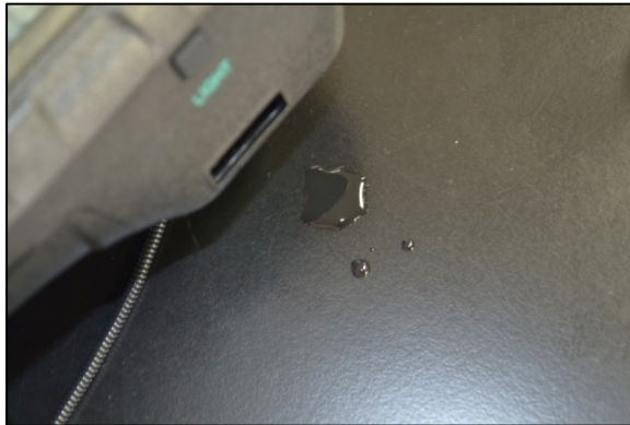
Figure 68. Saliva observed from the AquilaScan analyzer after leaking from the test cassette.
