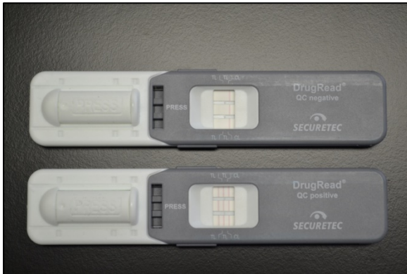
Figure 20. The DrugRead quality control cassettes. One negative control and one positive control.
