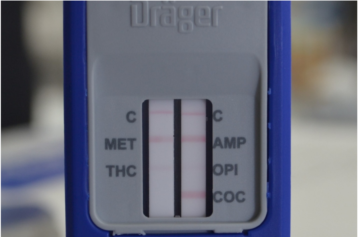
Figure 1. The faint negative THC line and not completely absent opiate line in an opiate positive sample. The presence of a line no matter how faint is considered a negative result with the DDC3000.
