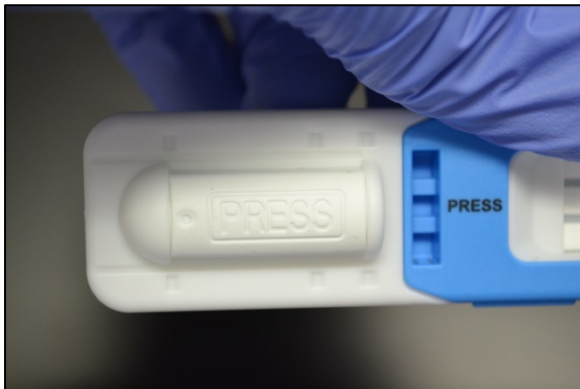
Figure 28. Once sampling is complete the collector is snapped back into the test cassette and an ampoule of buffer is manually broken.
