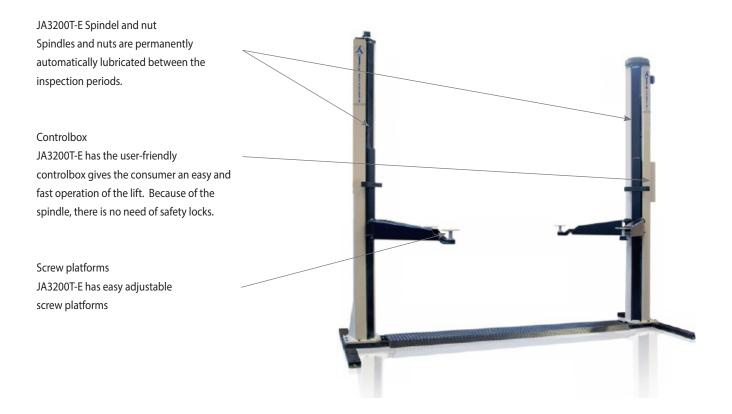
Jema Autolifte 2 post "Euro line" lift JA3200T-E has an amazing lifting height of 2000 mm which makes it a perfect workplace for event the tallest people. The JA3200T-E has asymetric posts which makes it easy to exit and enter the cars.
