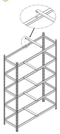
Step 3 - \*\*SRVS1896 & SRVS18126 ONLY\*\* Insert the shelf braces at each level. Shelf braces included in the 600D units only.
