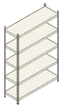
Step 5 - Complete assembly and move unit into place. For added stability shelving should be anchored to a wall - parts sold separately.
