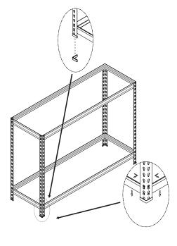
Step 1 - Start by joining a long beam and a short beam to an upright. Be sure to have the flat edge of the beams facing up. Repeat for each upright and attach the plastic end caps as shown. Create a second shelf level to join the upright halves.
