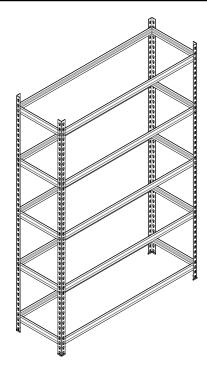
Step 2 - Complete the frame by adding the remaining uprights and adding shelf levels at desired height.\*
