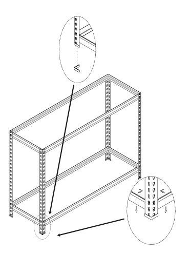
**Step 1** - Start by joining a long beam and a short beam to an upright. Be sure to have the flat edge of the beams facing up. Repeat for each upright and attach the plastic end caps as shown.
