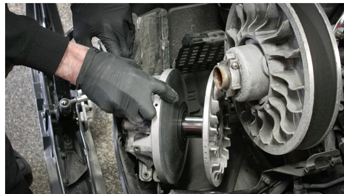
10 REMOVE THE PRIMARY CLUTCH USING THE SPECIFIC PULLER (PICTURE 10-11-12)
