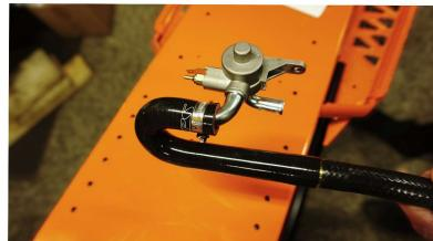
Step 4 - Drill a 1 inch hole in the plastic belly pan between the heat shield and the footrest to allow the hose to pass through. To ensure proper oil vapor evacuation the hose must extend beyon the belly pan by at least one inch
