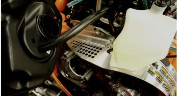
Step 3 - Plug the u-shaped end of the Precision EFI vent hose to the PCV valve, using the OEM clamp. Then follow the cables and the other hose down, right to the belly pan near the engine oil tank
