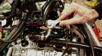
Step 2 - Remove the hose cooming from de PCV valve to the original air box
