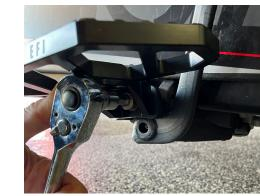
IN CONCLUSION, IT IS VERY IMPORTANT TO TIGHTEN THE ANGLE ADJUSTMENT BOLT AT 35 FOOT POUNDS.
