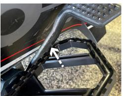
*IF YOU TRY TO DISENGAGE THE LATCH WHICH ALLOWS THE FLOORBOARD TO SLIDE FORWARDS AND BACKWARDS, IT WILL COME IN CONTACT WITH THE BRAKE PEDAL.*
