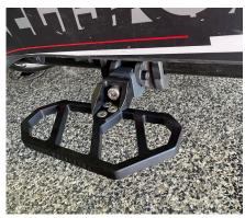
The best way is to unbolt the floorboard with a 8 mm allen key, then invert it (put it upside down)
