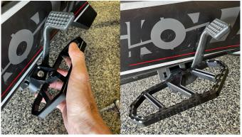
Lock the latch, flip the floorboard on the correct side and now choose the preferred angle.
