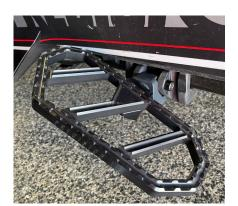
*Lock the latch, flip the floorboard on the correct side and now choose the preferred angle.*
