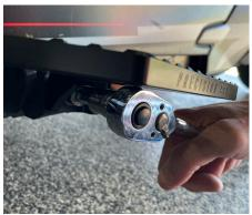
IN CONCLUSION, IT IS VERY IMPORTANT TO TIGHTEN THE ANGLE ADJUSTMENT BOLT AT 35 FOOT POUNDS.
