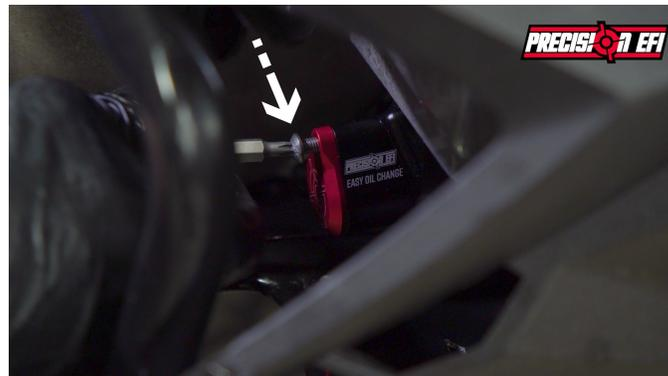
**2** RETIRER LA VIS AVEC LE MÊME TORX T25 QUE LE MARCHEPIED ET LE CAPUCHON FAIL SAFE PRÉCISION EFI
