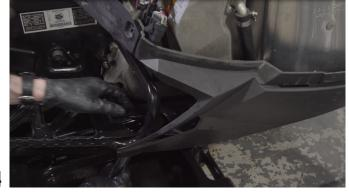
USE A DRAIN PAN UNDER THE FOOTBOARD, WE SUGGEST TO RAISE THE FRONT OF THE SNOWMOBILE BY AT LEAST 40 CM, BY USING SPACERS UNDER SKIS OR A CHAIN BLOCK, TO PREVENT OIL FROM SPREADING UNDER THE MUFFLER
