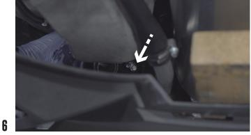
LOOSEN THE COLLAR AND REMOVE THE ELBOW
