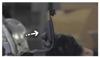
INSTALL THE FLOORBOARD STOPPER PLATE, MAKE SURE IT IS NOT DAMAGED OR BENT (LIKE THE IMAGE ABOVE) AND NOT INTERFERE WITH YOUR EASY OIL CHANGE.
