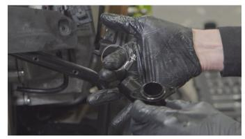
INSTALL THE COLLAR THEN INSERT THE NEW PART IN THE HOSE
