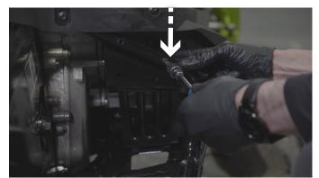
FOR YOUR NEXT OIL CHANGE, REMOVE THE FLOOR-BOARD STOPPER PLATE, SCREW
