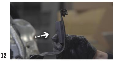
INSTALL THE FLOORBOARD STOPPER PLATE, MAKE SURE IT IS NOT DAMAGED OR BENT (LIKE THE IMAGE ABOVE) AND NOT INTERFERE WITH YOUR NEW PART
