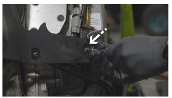
*Remove the right side cover and unscrew the body panel*
