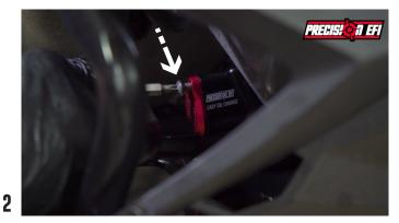
Remove with the same t25 torx , the easy oil change fail safe cap
