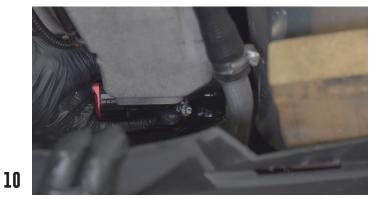
TIGHT THE COLLAR INSTALLED 3 MM FROM THE BEGINNING OF THE HOSE
