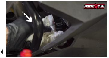
ONCE EMPTY, WIPE OFF OIL RESIDUE AND TIGHTEN THE INNER PLUG BY HAND AND PUT BACK THE PRECISION EFI FAIL SAFE CAP
