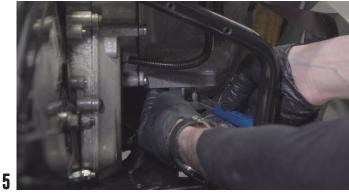
*Remove the 2 screws and the metal elbow under the oil tank (a minimum of 3 liters of oil will come out). Absorb the excess oil spilled on the belly pan*
