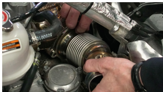
12 INSTALL THE PRECISION EFI DOWNPIPE, TORQUE FIRST AT 15 NM AND A LAST TIME TO 37 NM
