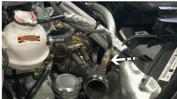
7 REMOVE THE SENSOR, BE SURE TO NOT TWIST THE WIRES
