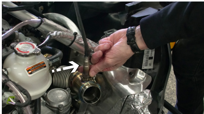
13 INSTALL THE SENSOR ON THE DOWNPIPE
