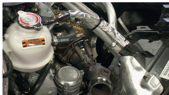
9 REMOVE THE COMPLETE DOWNPIPE, SPRING AND FLANGE.
