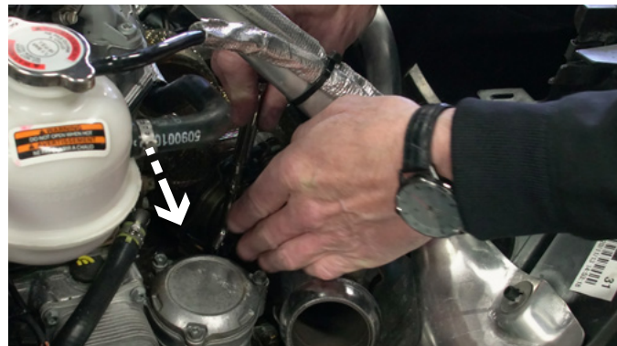
8 REMOVE THE BOLTS FROM THE DOWNPIPE
