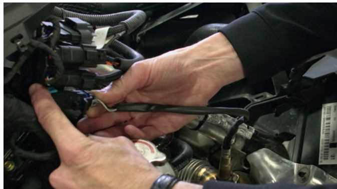
14 PLUG THE SENSOR CONNECTOR TO IS ORIGINAL LOCATION
