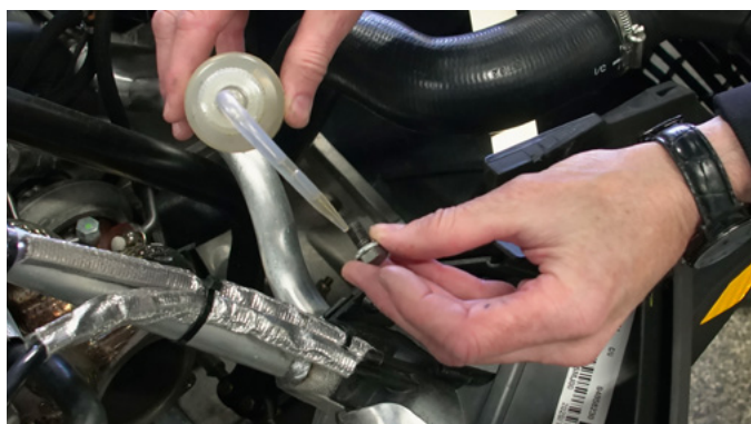
11 GENTLY LUBRICATE THE 3 DOWNPIPE BOLTS
