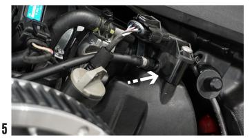
INSTALL THE SPACER BETWEEN THE INTAKE MANIFOLD AND THE MANIFOLD ABSOLUTE PRESSURE SENSOR WITH THE SCREW INCLUDED IN THE KIT, TAKING CARE TO TIGHTEN IT UNTIL ALL THE FLAT SURFACES ARE IN CONTACT.
