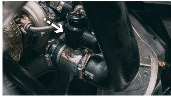
CONNECT THE BLOW OFF VALVE KIT TO THE TURBO OUTLET USING THE PROVIDED CLAMP.
