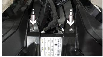
UNPLUG THE LIGHT CONNECTOR AND REMOVE HOOD BOLT DO NOT FORGET TO DISCONNECT THE FRONT LIGHTS AND THE OPTIONAL LIGHTS IF PRESENT.
