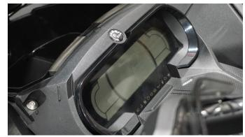
UNPLUG AND REMOVE THE INSTRUMENT PANEL
