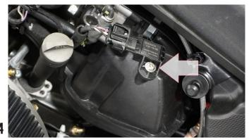
Then proceed to the installation of the Map Sensor Shim and hose supplied. Remove the Manifold absolute pressure sensor with a Torx T-30 screwdriver
