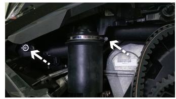
LOOSE THE AIR INTAKE TUBE CLAP AND REMOVE THE HOOD.
