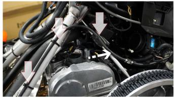
ATTACH THE VACUUM HOSE WITH THE ZIP TIES PROVIDED, TAKING CARE NOT TO TIGHTEN TOO HARD SO AS NOT TO OBSTRUCT THE PASSAGE.
