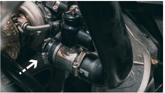
UNSCREW THE CLAMP AND DISCONNECT THE CHARGE TUBE CONNECTED TO THE TURBO OUTLET.
