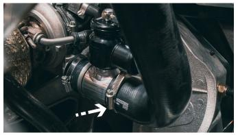
Connect the charge tube to the other end of the Blow Off Kit using the Oem Clamp.
