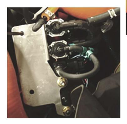
Step 3 - Remouve the red rubber plug from the back of the air box to connect the other end of the hose to this inlet (do not forget the clamp supplied)
