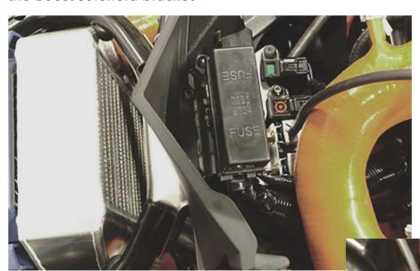
Step 2 - Connect the vent hose to the solenoid (do not forget the clamp supplied) and follow the same path as the blow off valve hose in direction of the air box
