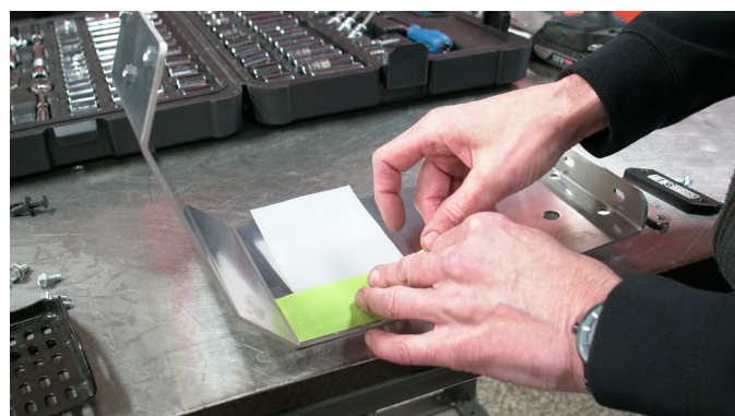
FOR EASY INSTALLATION AND PROTECT YOUR NEW PART AGAINST SCRATCHES, STICK THE SUPPLIED TEFLON SHEET ON THE INSIDE SURFACE USING MASKING TAPE.
