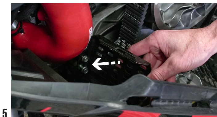
REMOVE THE UPPER CLUTCH GUARD BRACKET
