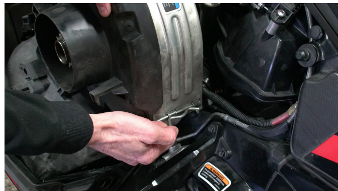
REMOVE THE UPPER CLUTCH GUARD.
