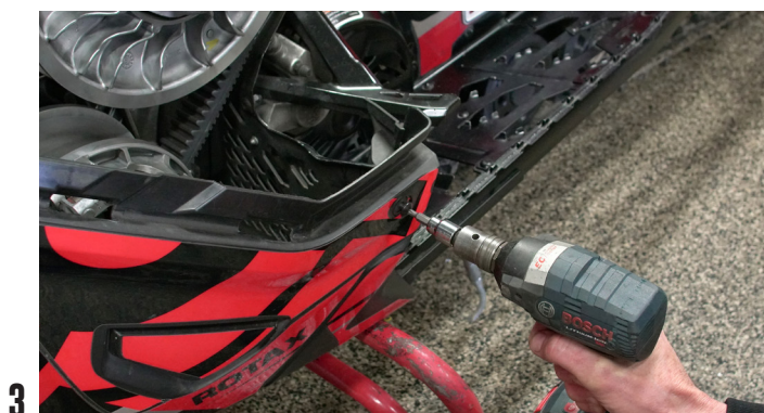
REMOVE THE SCREW ON THE SIDE PANEL.
