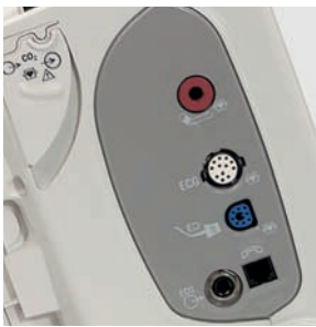
All monitoring connections are located on the left side panel. A carrying case pouch covers and protects ports and cable connectors from damage.
