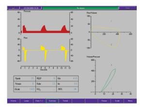
The **Summary** screen displays waveforms, loops and data on one screen.
