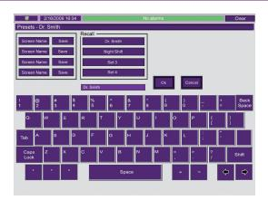
Touch **Save** to store the desired configuration, then select **Screen Name** and use the keyboard to label it.
