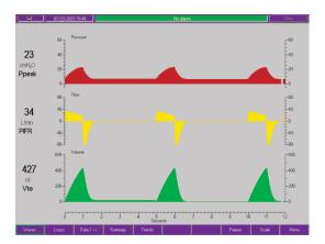
All selections and menu changes are done using the PalmTop monitor touch screen. Use the button bar at the bottom of the screen to select the screen to be displayed. The status bar at the top of the screen displays the alarm status of the ventilator, and the results and calculations from maneuvers performed.
