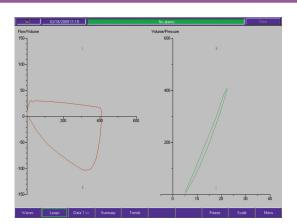
The **Loops** screen displays flow/volume and pressure volume loops. Options include the number of loops displayed and reference loops.
