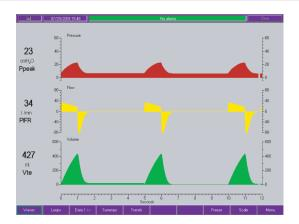
The **Waveforms** screen displays pressure, flow and volume graphics in real time. Digital values are displayed to the left of the screen and updated with each breath.
