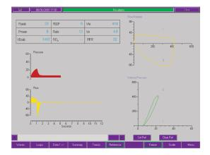
Using the cursors on a frozen waveforms screen, you can select a breath to store as a reference breath. Frame the desired breath with the cursors and select the **Reference** button to store the breath as a reference.
