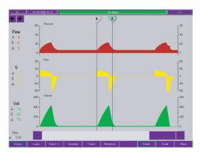
When the **Waveforms** screen is frozen, cursors appear. Touch the cursor to select it, then touch the location to place the cursor. Scroll arrows allow fine movement of cursors. Breath data at the left of the screen displays the values at the points of the cursors and the delta difference between them.
