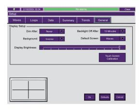
Touch **Menu**, then **Setup**, then the **General** button to calibrate the touch screen and configure the display setup. The PalmTop monitor is powered by the docking station. To turn the display off, select **Backlight Off After** and select immediate or the desired number of minutes. The display will become active again if the touch screen is touched.
