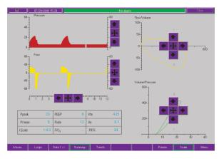
Touch the **Scale** button to change scales. The outside arrows allow manual scale change. Touch the center arrows to auto scale.
