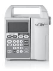
The ACCLAIM Encore™ Infusion System is a peristaltic pump that utilizes standard Hospira gravity sets. The pump is a simple, easy-to-use, standard tubing device. This device can be used across the healthcare continuum in the hospital and alternate site areas, including the home care environment.
