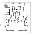
If available, route the Top Tether strap to the appropriate anchor and connect. Do not tighten until car seat is installed (See pages 47 for Top Tether installation instructions).
