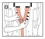
**Important:** Make sure loop ends of **BOTH** straps are threaded completely onto the arm of the metal hook. Attach left harness first then right harness, while looking at the back of the car seat.
