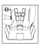
If available, route the Top Tether strap to the appropriate anchor and connect. Do not tighten until car seat is installed (See pages 47 for Top Tether installation instructions).
