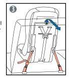
Slide the SuperLATCH™ through the opening above the forwardfacing belt path label which is on the side middle portion of the car seat. Be sure the SuperLATCH™ strap is flat and not twisted. Adjustment strap should be on the child's left side of the car seat.
