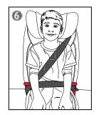
Place shoulder belt portion so that belt lays properly across child's collarbone, interior to the shoulder. Use the upper belt guide on the headrest to properly position the shoulder belt).
