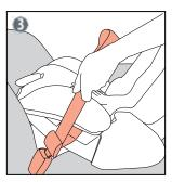
Tip: If available, add rear-facing top tether connector strap to appropriate anchorage and attach top tether strap (See page 37 for installation instructions).
