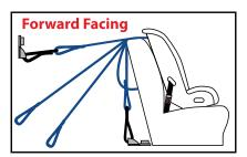
**Important:** Diagram shows a variety of places you might find a top tether anchor. Consult vehicle manual to locate correct anchor.
