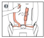
From back of car seat, re-attach shoulder straps to metal hook (left strap first).
