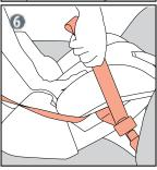
**Tip:** If available, add the rear-facing top tether connector strap to the appropriate anchorage and attach the top tether strap (*See page 37 for installation instructions*).
