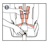
From front of car seat, pull shoulder straps out and re-thread them through the correct height harness slots.
