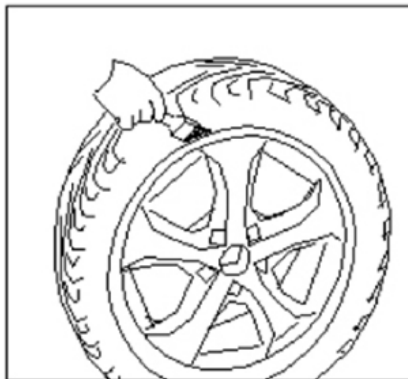
Applying lube after breaking
