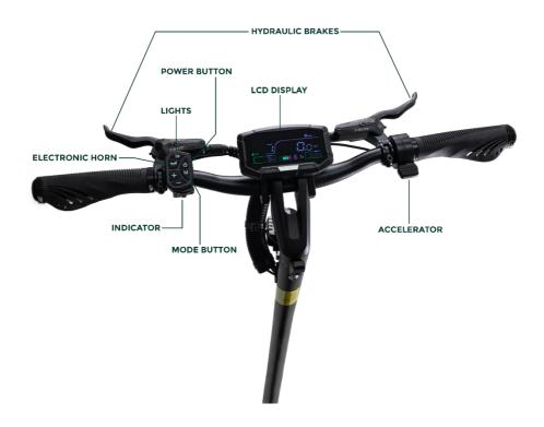
2.3) To power up the G2 Pro Max Electric Scooter press and hold the on / off button on the Smart User Controls Panel.
