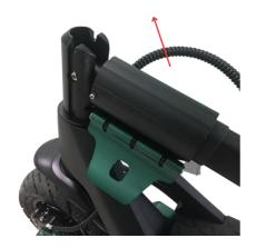
Once unfolded, use the **Stem Clamp** to hold the stem in place. Ensure this is fully tightened. See below.
