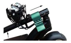
Once unfolded, slide the stem clamp down oven the folding mechanism, ensure the stem clamp is sitting flush to the bottom See below.
