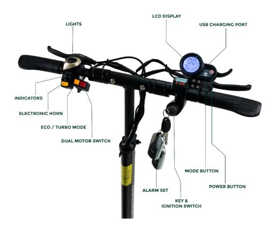
2.3) To power up the P1+ Electric Scooter, firstly turn the eScooter on from the on / off button on the base. Ensure the ignition key is fully turned to the right (clockwise) or the key fob ignition button has been pressed twice. Once the ignition is switched on or the key fob ignition button has been pressed twice proceed to hold the power button to turn on the P1+ Electric Scooter.
