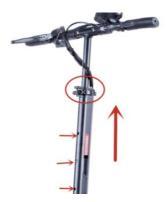
4.2.1) Your stem lever may need to be adjusted over time, to adjust your stem lever tension use a 10mm spanner and adjust the stem bolt. See below.
