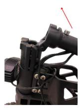
Once unfolded, use the **Stem Lock Screw** to hold the stem in place. Ensure this is fully tightened. See below.
