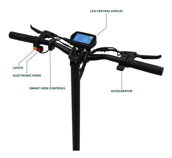
2.3) To power up the G2 Pro Electric Scooter, ensure the ignition key is fully **turned to the right (clockwise)**, then **press and hold the on / off button** on the **Smart User Controls Panel** to turn on the G2 Pro Electric Scooter.
