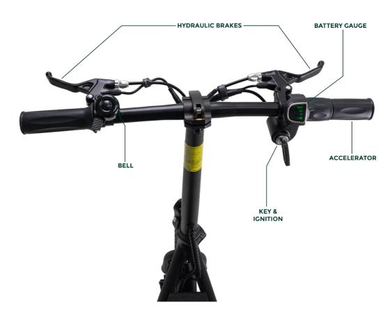
2.3) To power up the Electric Carry Commuter Scooter **turn the ignition key clockwise**.
