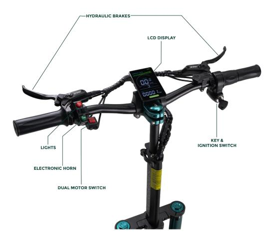
2.3) To power up the EVR Pro Electric Scooter, firstly turn the eScooter on from the **on / off button on the base**. Then ensure the ignition key is fully **turned to the right (clockwise)** or the key fob ignition button has been **pressed twice**. Once the ignition is switched on or the key fob ignition button has been **pressed twice** the eScooter will power up.
