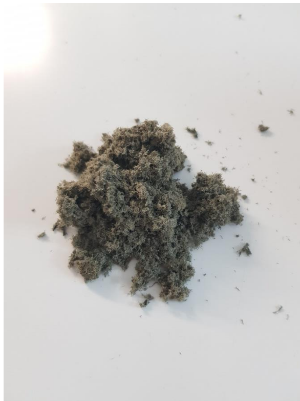
Figure 2: Sample 2 ground for ISO 20136 testing
