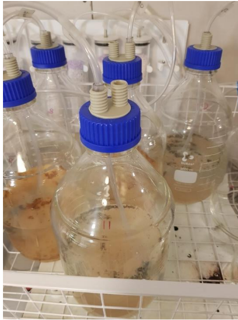
Figure 3: Reactors in shaker with CO 2 free air supply.
