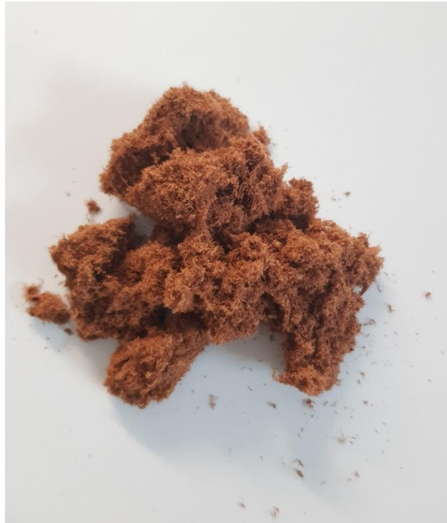
Figure 1: Sample 1 ground for ISO 20136 testing
