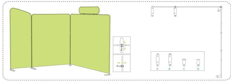
3 Put the clip between two frames and fix it with screw, we have four kinds of metal bases (A,B,C,D).
