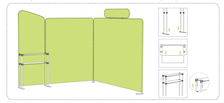
4 Put the aluminum tube of layer board on the metal bases, then Install the shelf boards. Finally fix it with screw. Finish.
