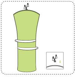
Fit both lights on the top and run the electric cords inside the graphic.
