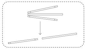
2 Assemble the hardware, connect all the aluminum tubes together, they are all are corded.
