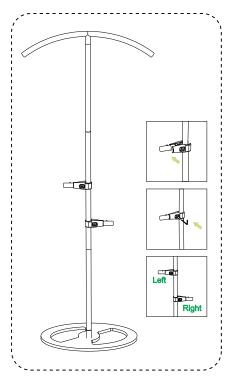
4 Assemble the handle clip corded as shown, and use hexagonal key to fix it.
