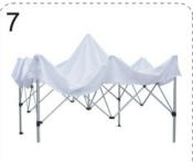
Lift inside pole in center to extend frame completely
