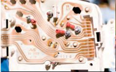
Here's a look at the back side of the cluster with all the hardware in. Starting at the center top position and going clockwise we have the upper tach stud, positive terminal, Ignitor terminal, bottom stud and ground terminal. Now it's time to connect the wires to the eye connectors. connectors.
