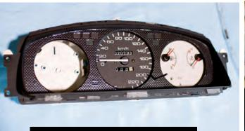
With the circuit board peeled back flip the cluster back over so we can see the front and reinstall the back portion of the cover. We'll need this in place so we can mock up our tach fitment.
