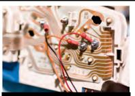
Here's a look at all the wires mated to the connectors. Make sure to do a quick pull test to insure that they are properly secured.
