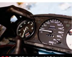
Now that the terminals are installed we can throw the cover backing on and mount the tach.
