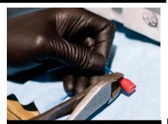
27 Now it's time to take care of that pesky blue wire we have left over. This is for the supplied switch that allows you to configure the tach and display peak RPM. I decided to add a spade connector between the cluster side and switch side to make installation/removal an easier
