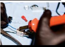
On one side of the switch we have the blue wire coming from the tach and on the other I used some of the left over black wire for the ground side. I decided to solder them in but you can use the supplied spade connectors for this.
