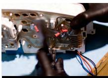
With the tach in place use the supplied washers and 7mm lock nuts to secure the tach to the cluster. I had to leave the lower corner of the circuit board disconnected to secure the lower stud, but the top stud went right through an already existing hole – score! (That's what she said.)
