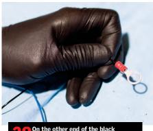
29 On the other end of the black wire I installed the supplied large eye connector for the ground.
