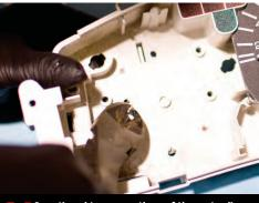
16 I continued to remove three of the protruding pegs where I am going to run hardware so that the bolt heads aren't limiting the mounting depth.
