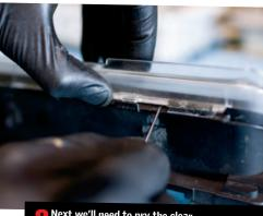
Next we'll need to pry the clear portion of the cover off the backing. Be extremely careful to work slowly so you don't crack the cover. The idea is to break all the small glued areas without damaging the screen. Fortunately for me the previous owner of this cluster already performed this task when they installed the faux-carbon overlay.
