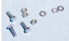
Here is the hardware that is going to be used to connect the tach wiring directly into the circuit board. You can pick these up at most any hardware store: (3) 4mmX7 nuts, (3) 4mmX7 bolts and (3) 4mm washers.
