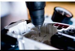
Now pull the tach back out and remove the cover so you can drill your spots. Make sure the circuit board is out of the way before you start drilling! I used a very small drill bit to start the holes since I wasn't sure if the placement would clear the circuit board or not. It's a good idea for you to do the same since there is some guess-and-check involved in this install.
