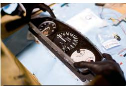
Once everything is installed and you're positive you don't need to make any further adjustments we can glue the clear screen back onto the cover. Using super glue, place a couple dots along the areas where the screen was originally attached and firmly hold the cover in place as it dries. Don't forget to reinstall the cluster bulbs.
