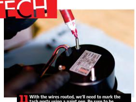
With the wires routed, we'll need to mark the tach posts using a paint pen. Be sure to be thorough with your paint coverage since the idea is to leave two dots on the plastic where the posts will go
