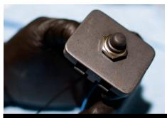
Last but not least you'll need to decide where you want to install your switch. I decided to use the vacant plate on the left side of the EG dash under the dimmer switch. I removed the plate for drilling and installation because it's a lot easier to work on a table than crawling around inside a car.
