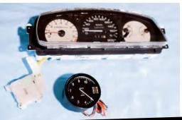
Here's a look at the EG Civic cluster I'll be working on and the STACK ST200. Ignore the white box and wires at the bottom of the cluster – unless you also have a JDM unit with door indicators this piece shouldn't be on your cluster anyway
