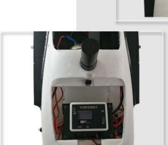
The PPK antenna is reserved to facilitate carrying the PPK module to improve the POS positioning accuracy
