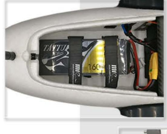
The battery cabin can accommodate 6S@16000 / 22000 mah batteries
