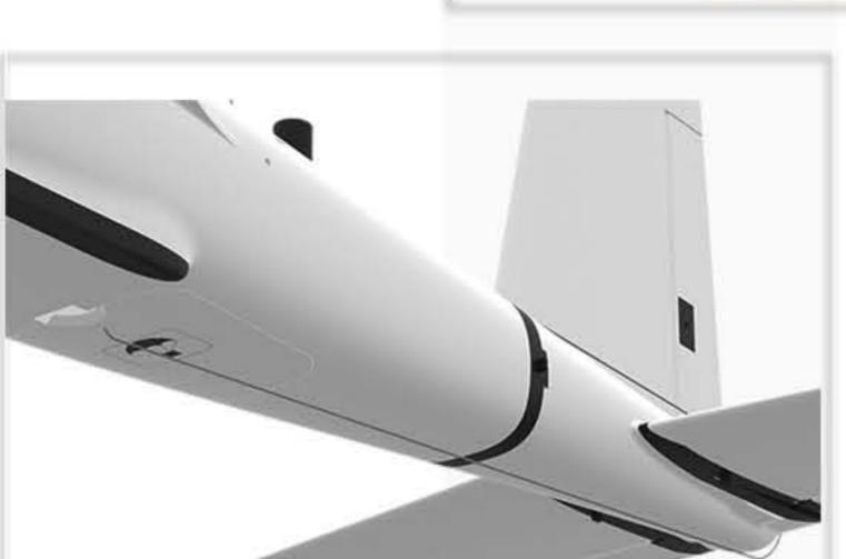
The size of the parachute cabin is 172 × 113 × 52mm, which can easily place 6-8kg parachute
