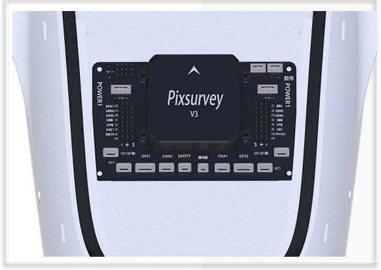
The open platform design of the flight control cabin facilitates the installation of open source /commercial flight control installation
