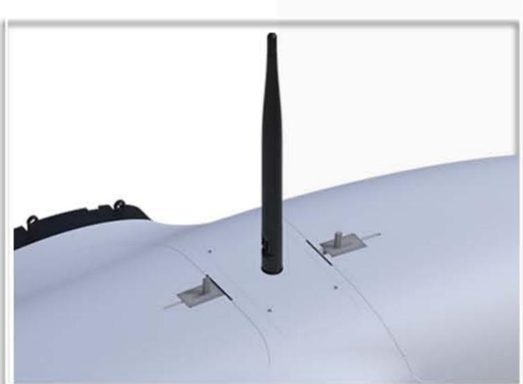
The distribution cabin cover is reserved with data transmission antenna holes, which is convenient for the assembly and disassembly of the antenna
