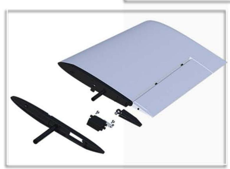
Horizontal tail servos do not need to be buried in advance, which is convenient for servo maintenance
