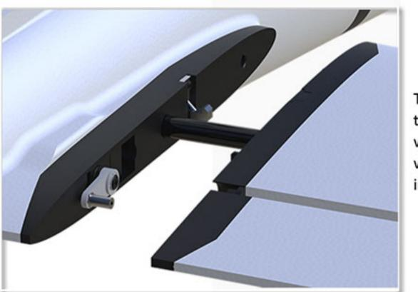
The horizontal tail adopts a tool-less quick-release structure, which is automatically locked when it is pushed and pulled out immediately when pressed The left and right horizontal tails are designed with independent control of dual servo. Even if one side fails, the aircraft can return, which improves the safety of the aircraft
