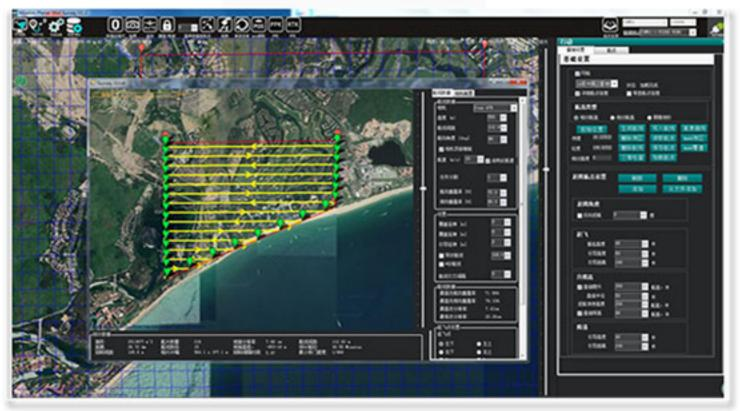
Mission Planner Vtol Survey ground station is based on Mission Planer, which is deeply optimized according to the characteristics of aerial survey operations. It is concise and efficient, and is suitable for new users to get start quickly
