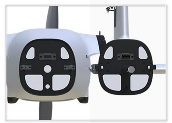
The vertical tail and fuselage adopt a 5-point integrated toolless quick-release structure
