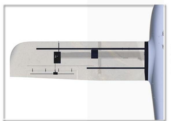
φ12×1000mm Outer covering φ14×560mm Main carbon tube φ12×600mm Auxiliary carbon tube Ensure the overall rigidity of the wing. The wing and fuselage with the embedded box structure enhance the contortion resistance of the wing
