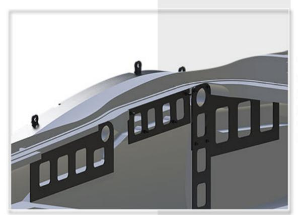
The inside of the fuselage is equipped with a wire groove and a removable baffle, which is matched with nylon braided sleeves to ensure simple and efficient wiring in the cabin
