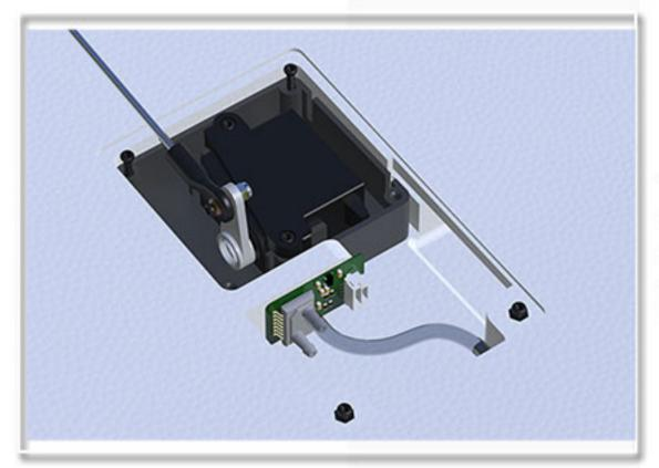
The aileron servo cabin not only facilitates replacing servo, but also can be equipped with an airspeed meter module to improve the airspeed detection accuracy
