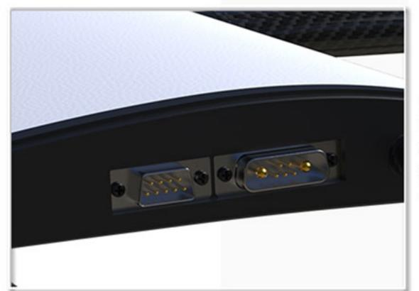
Dual connector can realize signal line redundancy, improve system stability, reduce wiring difficulty, and is compatible with 4 + 2 layout The wing wiring cabin facilitates the installation of power signal cables. With the wiring board, the wing power system can be quickly disassembled and assembled
