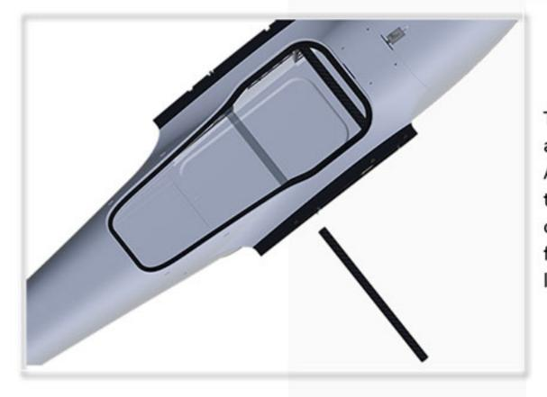
The auxiliary carbon tube adopts a toolless quick-release design. After disassembly, it can open the main and auxiliary cabin. It can be equipped with a five-lens full-frame tilt camera or a 1.5kg lightweight lidar
