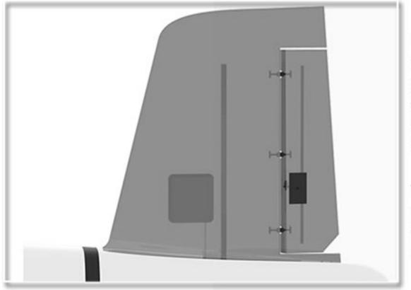
Embedded carbon tubes on the vertical tail rudder surface increase the strength of rudder surface, increase the rudder angle fixing plate, and increase the rudder surface response speed
