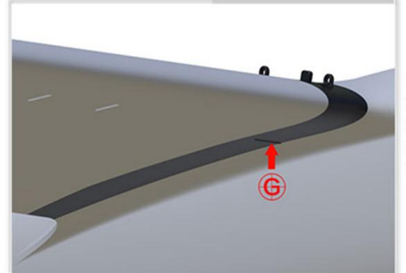
The center of gravity of the aircraft is under the raised position of fuselage hook and the wing root plastic (same position)
