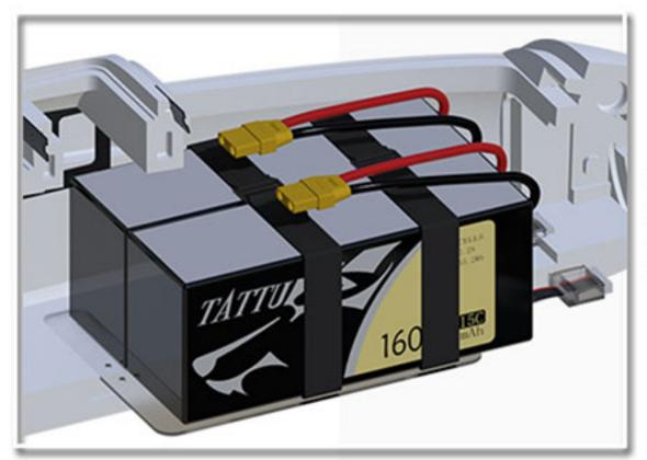
Battery cabin supports 2 6S@16000 / 22000mAh(Li-Po) whitch provides strong power for long endurance
