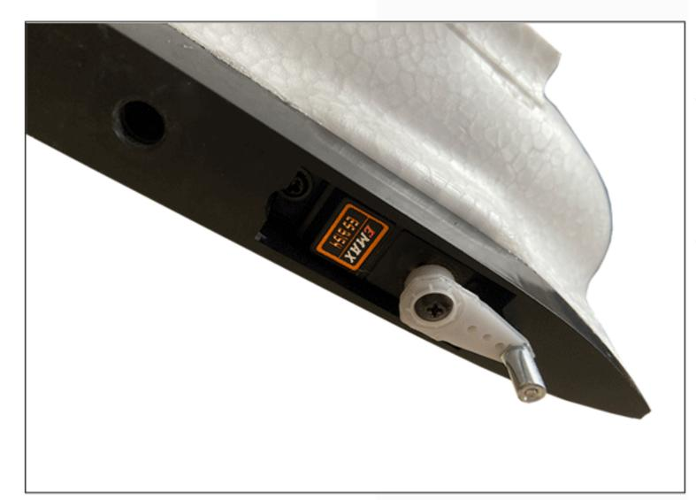
The horizontal tail servo does not need to be embedded in advance, which is convenient for the replace of the servo.
