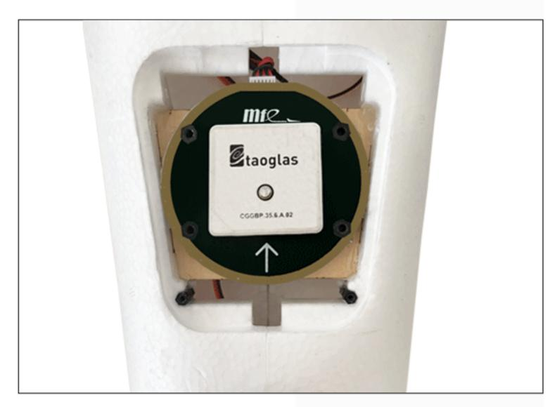
The GPS cabin is located at the rear of the fuselage, the size of 78×58×37 mm can place the GPS and compass module, and the electromagnetic environment is clean.
