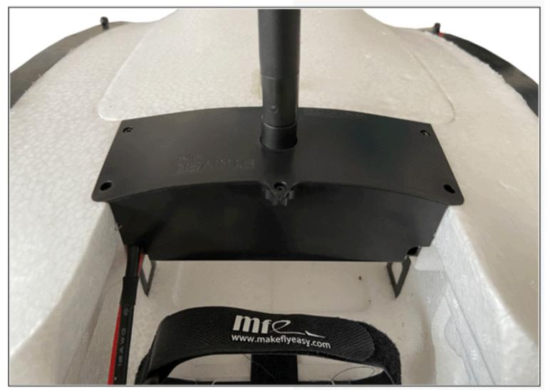
The power distribution compartment is made of injection molded engineering plastic, improve the structural strength of the fuselage.
