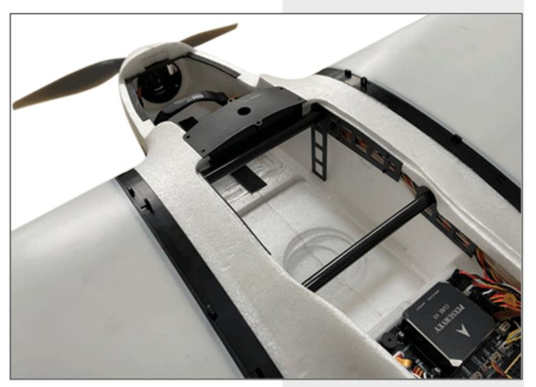
Large amounts of high-strength lightweight carbon fiber, wood board, and PC board are used in materials.
