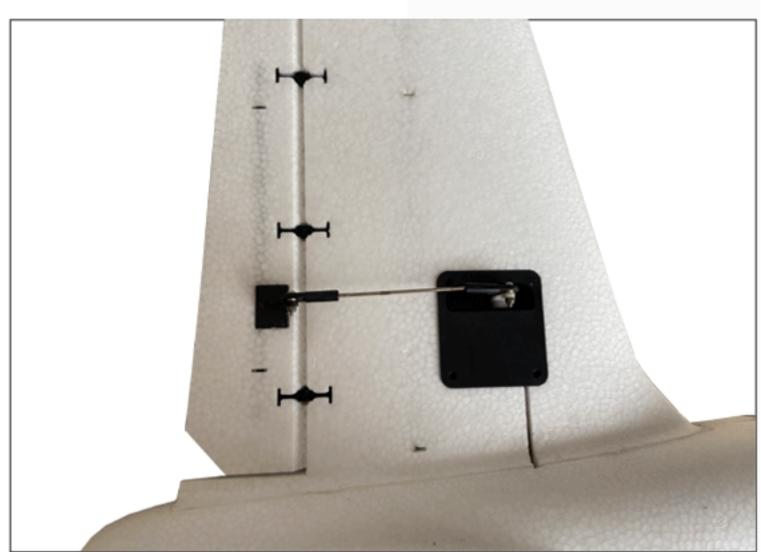
The vertical tail servo can be flexibly disassembled and assembled for easy maintenance and replacement.
