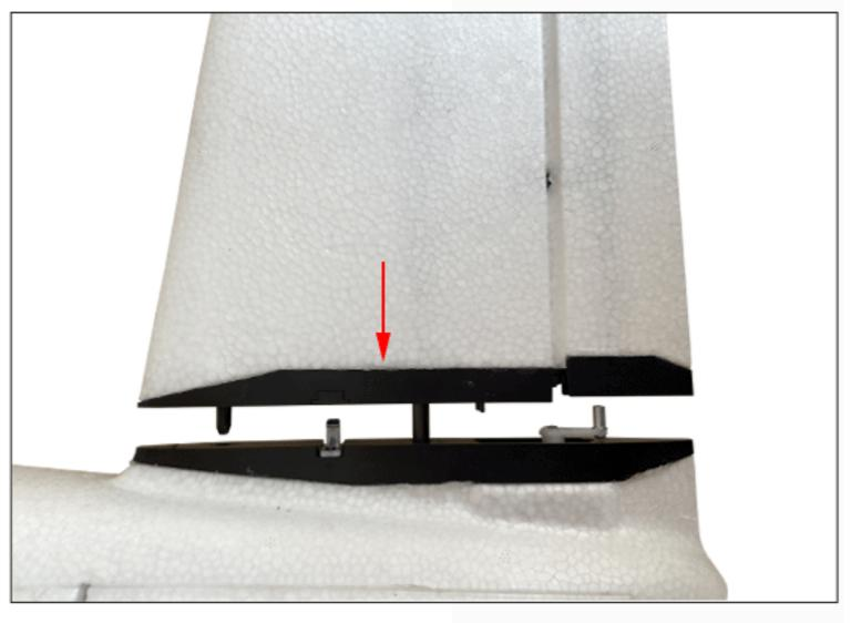
The horizontal tail adopts a toolless quick-release structure, which is automatically locked with one push and pulled out immediately with one push.
