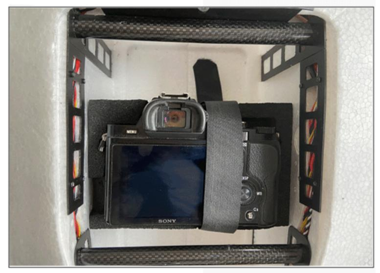
Load compartment size. 220×150 ×110mm. Can hold Sony A7R series cameras and five-lens tilt camera.
