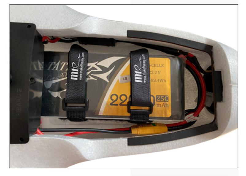
The battery ties have a reasonable layout, which is convenient for binding and unbinding, and effectively avoids entanglement.
