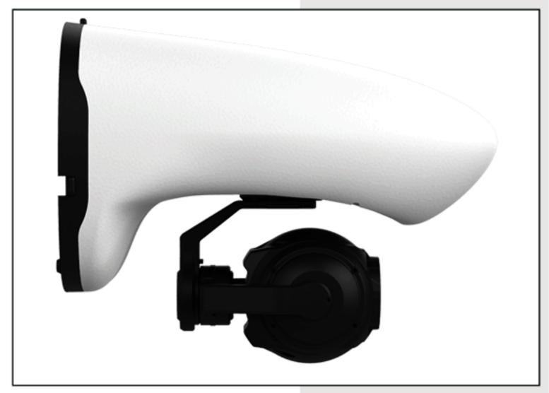
The design file of the nose cabin is open source, and users can customize the mounting plate according to the installation hole position of the pod.
