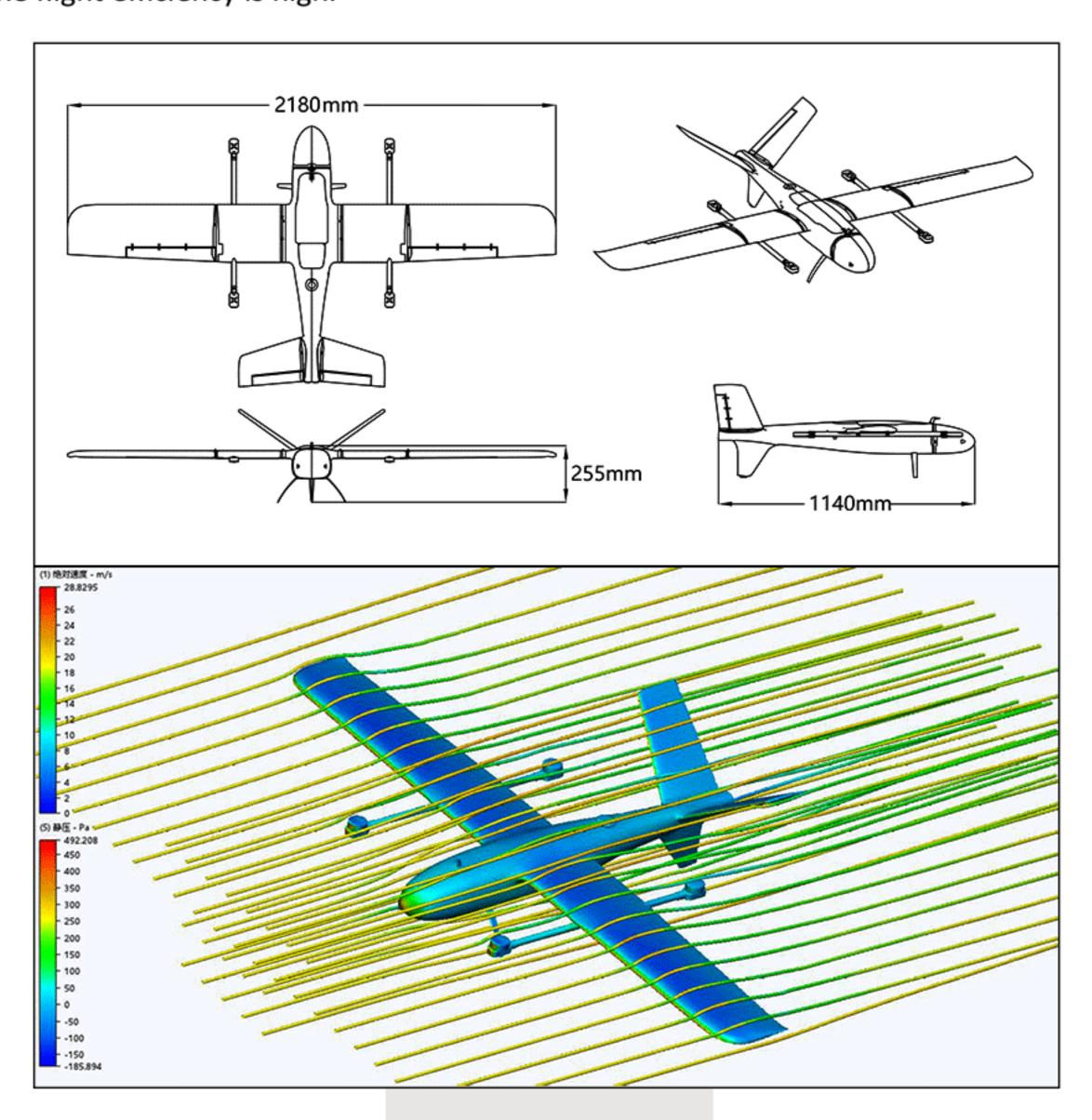
The Hero VTOL adopts a streamlined shape as a whole to reduce flight resistance as much as possible while ensuring stable flight.
