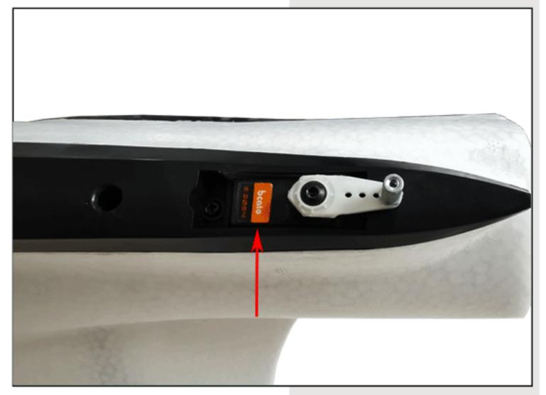
The tail servo does not need to be pre-embedded for easy maintenance.
