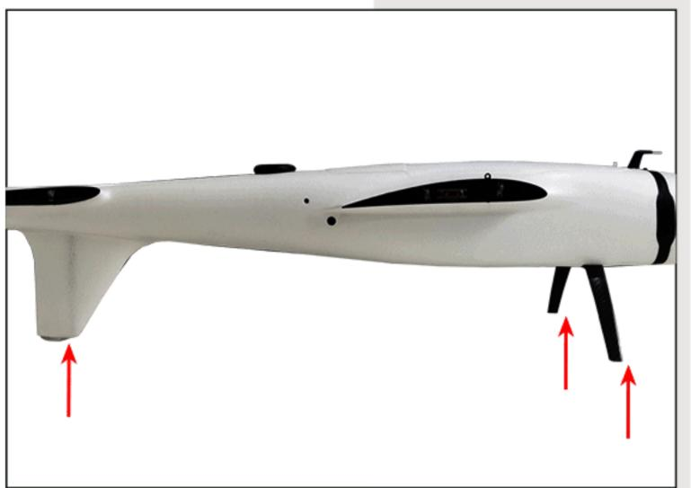
The bottom of the fuselage adopts the rear three-point landing gear, with high ground clearance, large mounting space, and the tail rotor does not touch the ground.
