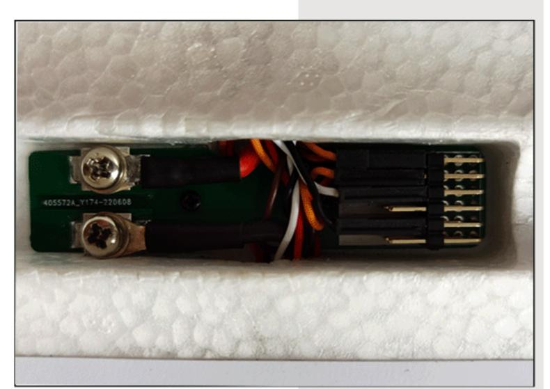
(Optional) Wiring board Quick-release wing power system
