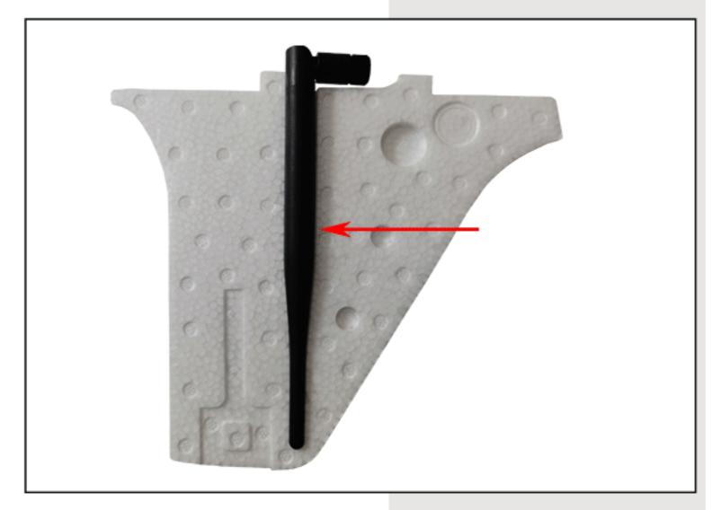
The 195mm rat tail glue stick antenna can be pre-buried in the vertical tail, which not only improves the support strength of the vertical tail, but also has a clean electromagnetic environment and
