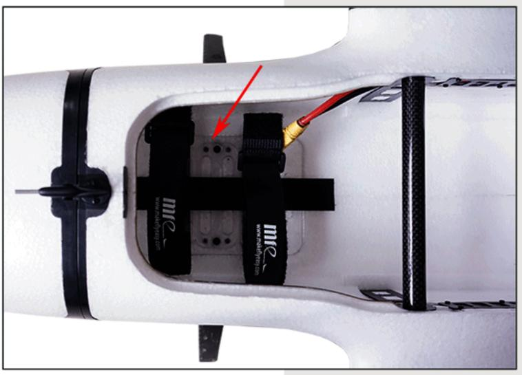
The size of the battery compartment is 326\*110\*78mm, and the maximum support is 6S@30000mah solid-state lithium battery.
