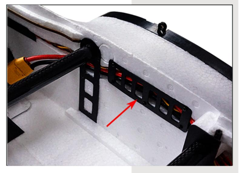
The inner side of the fuselage is designed with wire grooves and removable baffles to facilitate the installation of wires, and the wiring in the cabin is simple and efficient.
