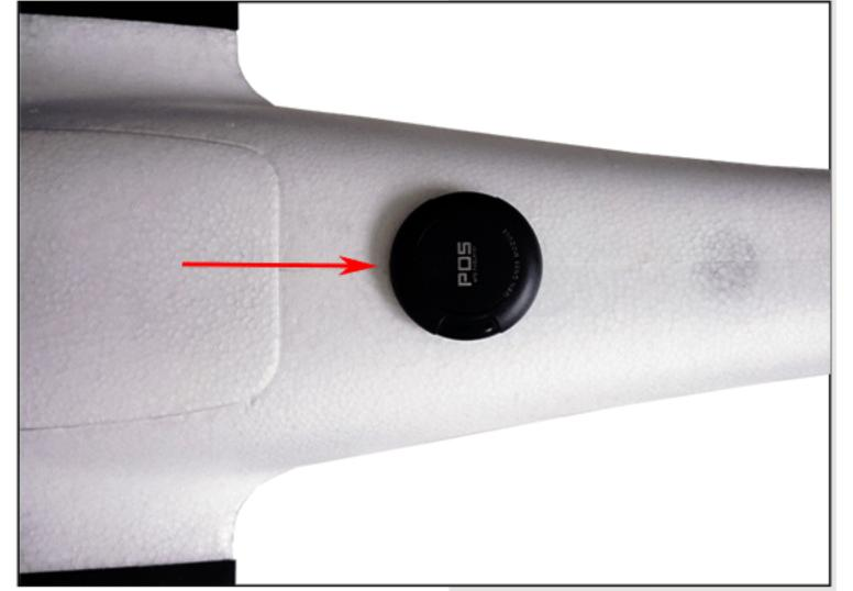
The GPS and compass modules are placed above and behind the flight control cabin, and the electromagnetic environment is clean.
