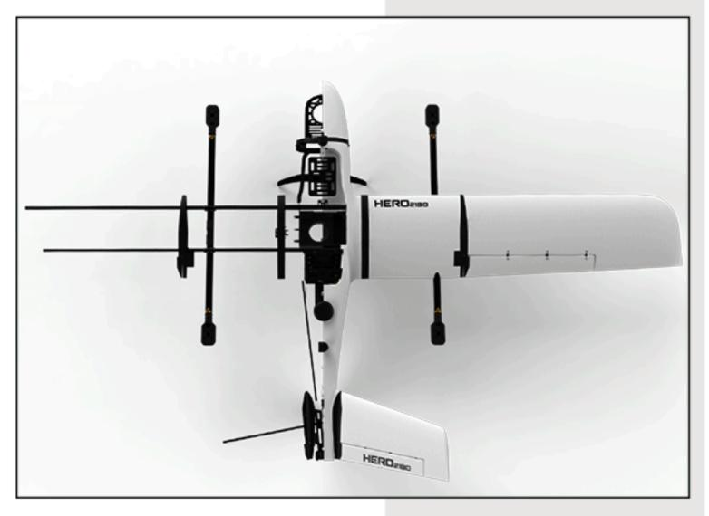
A large number of high-strength and light-weight carbon fibers, wooden boards and PC boards are used in the materials.
