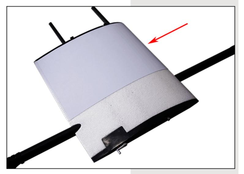
The surface of the wing root section is reinforced with 3M stickers, which enhances the rigidity of the aircraft and improves the torsion resistance of the wing.
