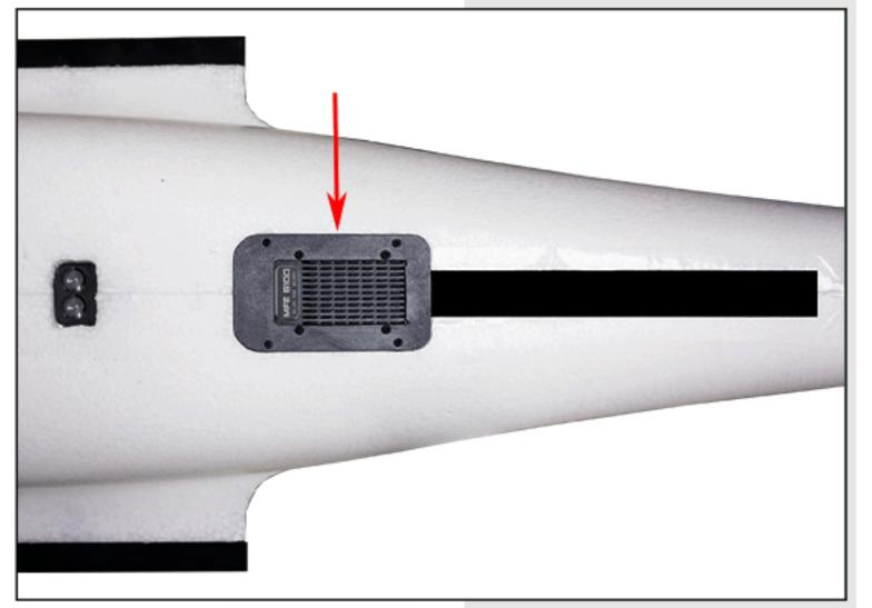
The tail push ESC is placed under the rear of the flight control cabin, with an external aluminum shell, which has a good heat dissipation effect.
