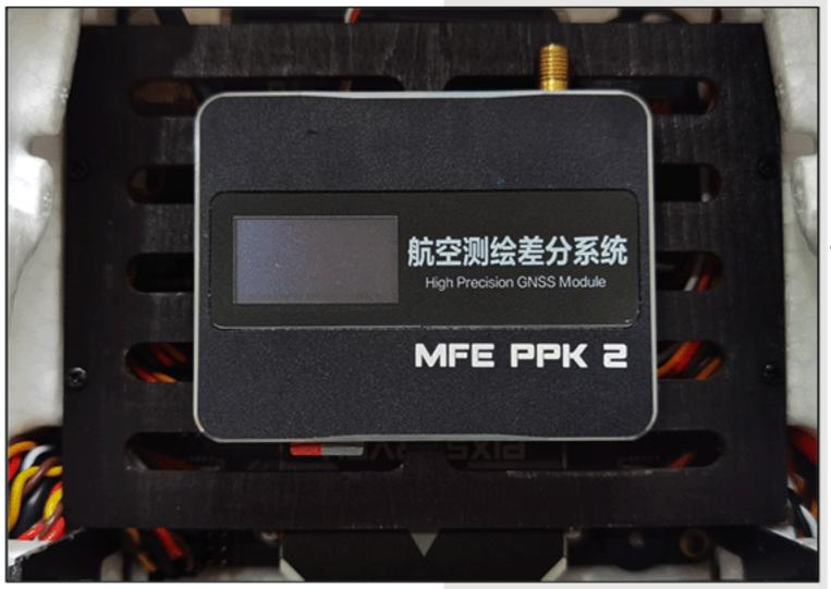
The top layer can install PPK or image transmission equipment.
