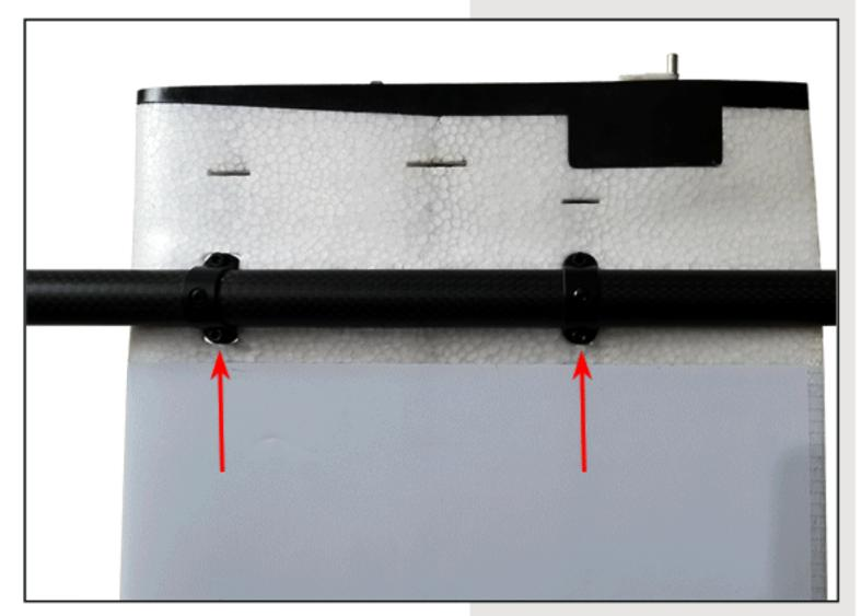
The VTOL Rotor Arm is fixed by an aluminum alloy wrapping structure, which can be installed and removed as a whole for easy maintenance.
