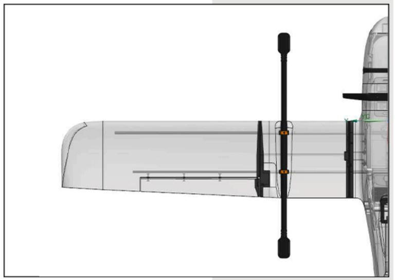
The wing is composed of main carbon tubes, auxiliary carbon tubes, vertical arms, and plastic parts to form a frame structure to improve the overall strength.
