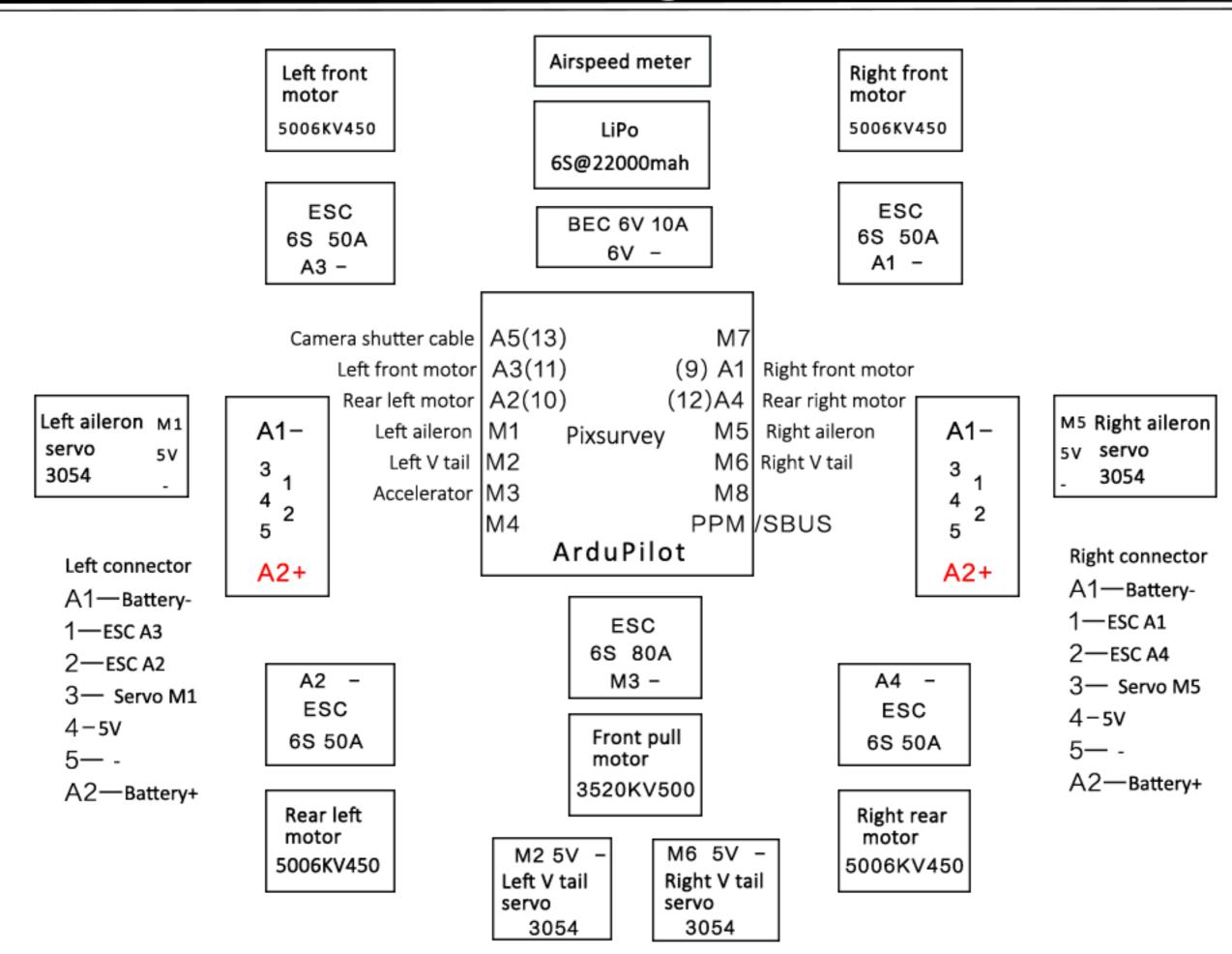
Note: Before powering on, be sure to check the connector line sequence one by one to prevent short circuit.
