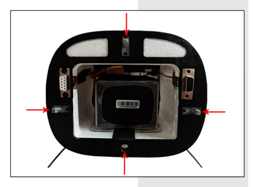
The nose cabin adopts a four-point connection structure, which is stable and reliable and supports quick release.
