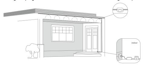
The adapter and controller, for safety, durability and aesthetic reasons, are designed to be extended for indoor installation and are therefore not waterproof. Please ensure controller and adapter are shielded from water if you plan to place them outdoor. You may contact customer service at support@eufy.com for a waterproof box solution.
