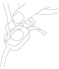
4. Peel the VHB adhesive from the back of each light, then firmly press the light against the surface for at
