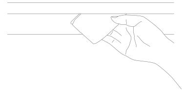
2. For the best wall-washing effect, the light string should be installed 2-4 inches (5-10 cm) away from the wall surface. Use the provided positioning card for measurement.
