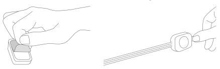
5. In extremely hot/cold or humid environments, it is strongly recommended to use a cable clip and screw to secure between every two lights.
