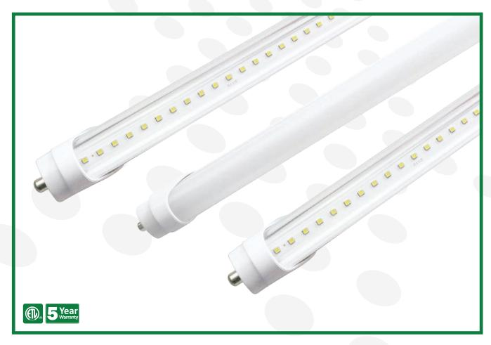
Our new ZELL T8 8 FT Tube offers significant energy efficiency and lifetime improvements over fluorescent lamps. Zell is made of full Aluminum housing with PC Cover lens which makes Zell the most durable 8 FT tube of its kind. Our ZELL lamps are installed by bypassing existing fluorescent ballasts and hard-wiring tombstone lamp-holders directly to incoming AC power leads. Dual-ended bypass lamps eliminate the need to replace shunted tombstone lamp-holders in existing fluorescent luminaires.
