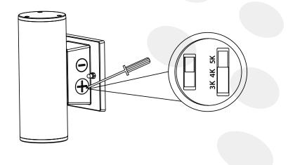
Note:Please turn off the power before adjusting the wattage and CCT. CCT adjustable instruction fixture.
