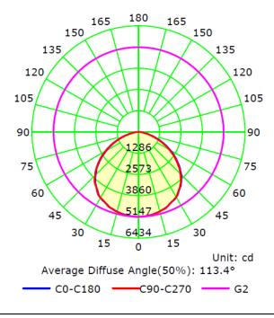
Longitudinal Classification: Very Short Measurement Flux: 14866.5 lm Downward Ratio: 100% Luminaire Efficacy Rating (LER): 102.18 Max. Intensity: 5147.31 cd
