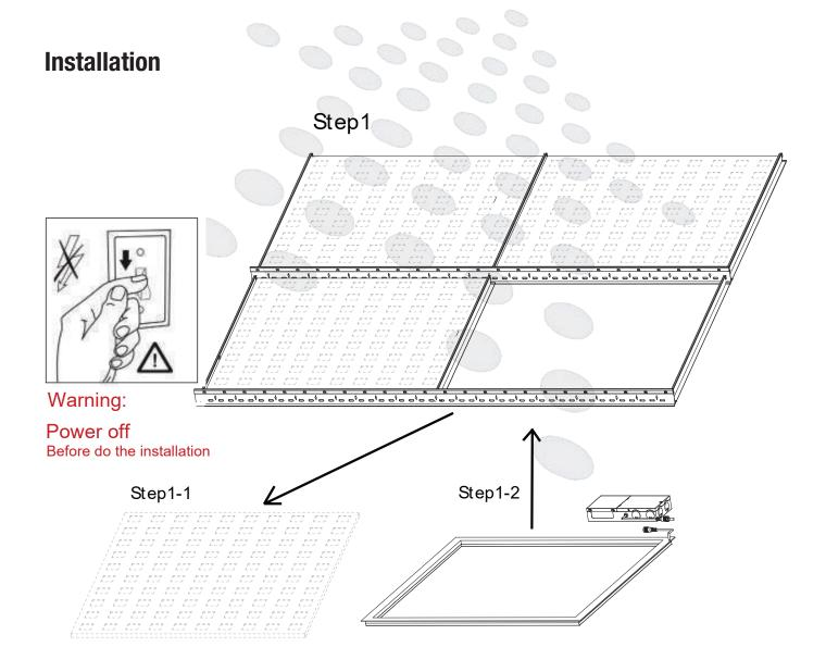
Step 1: Make sure of all the power is off before installing. Remove the one ceiling tile that you need to install light fixture on. Then place the light fixture on the T-bar carefully and make sure it is correctly in place and secure.
