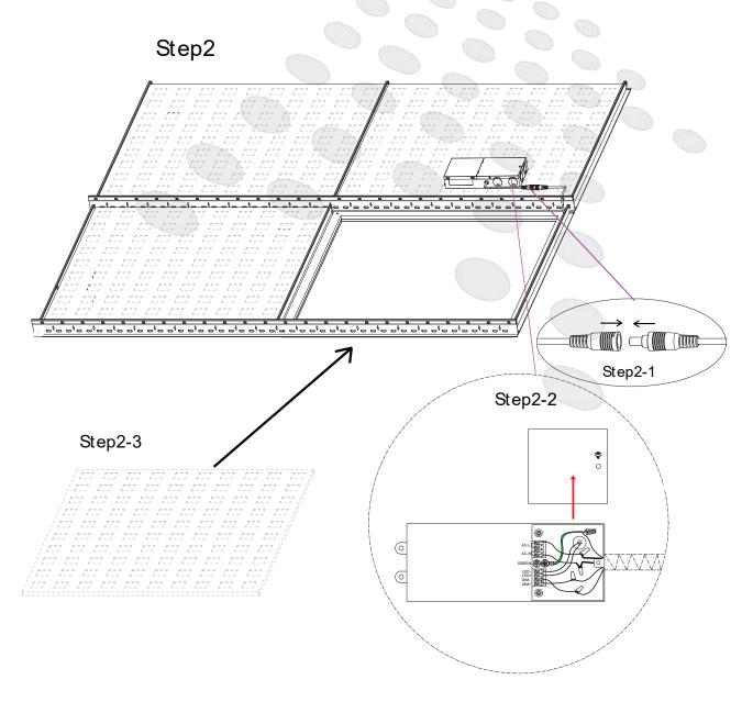
Step 2: Place the driver on top of the next ceiling tile. Connect the cable between the driver and the lighting fixture.
